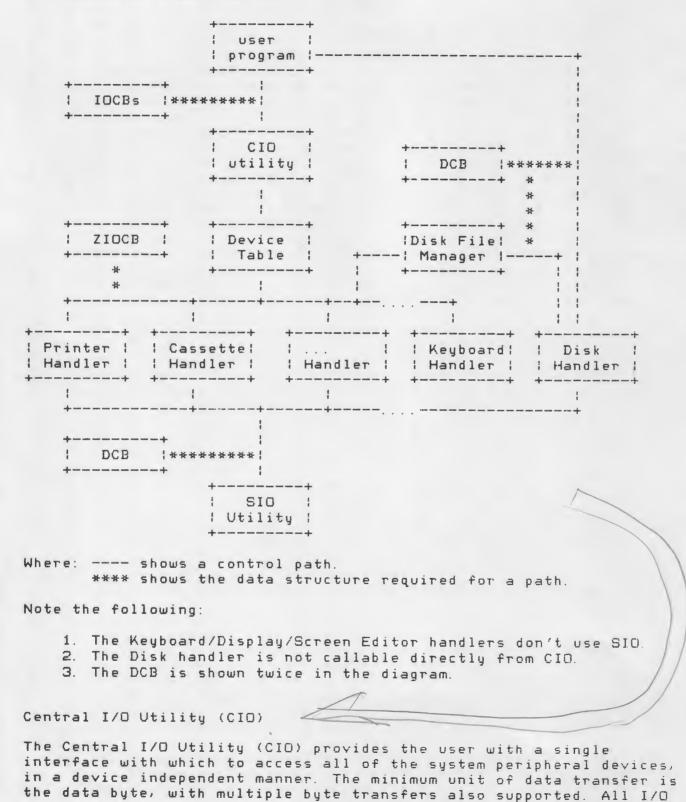
operations are performed on a "return to user when complete" basis; there is no way to initiate concurrent "overlapped" I/O processes.
