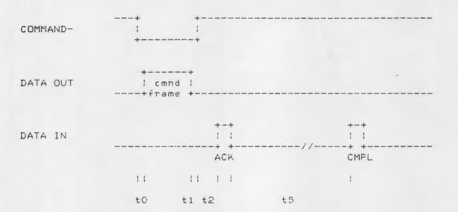
tO is the delay between the lowering of COMMAND- and the transmission of the first byte of the command frame. The computer generates this delay.
