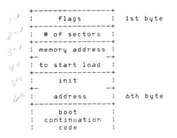
The 1st byte is stored in DFLAGS [0240], but is otherwise unused. It should equal zero.
