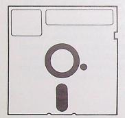
The small hole is an index mark which enables the disk drive to reference the disk correctly.
