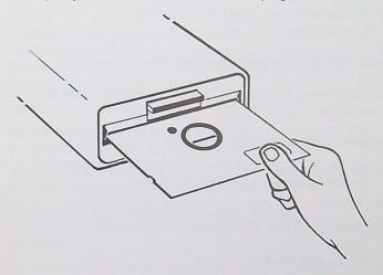
If you have a single disk drive, insert your system disk into it. The system disk is the one provided with the disk drive and documentation, and which contains the information needed to make your disk system work correctly. If you have a dual disk drive, insert the system disk into the left-hand (or topmost) drive (Drive A).
